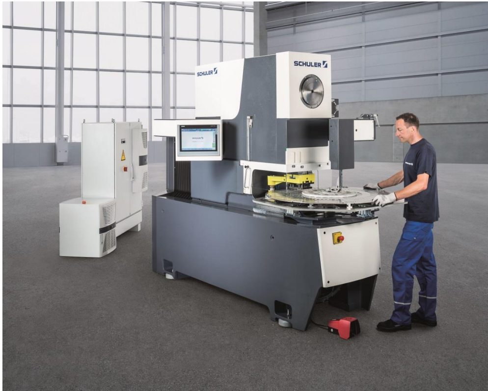
▲ The new Performer S produces laminations for electric motors and generators with diameters of 80 to 1,800 millimeters.
